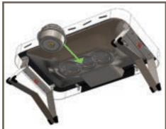
3. To fit the EcoBurner, first light the EcoBurner as normal. The burner head should be glowing orange before the EcoBurner is positioned. Align the EcoBurner with the Spring Clip cradle and push firmly into place.
