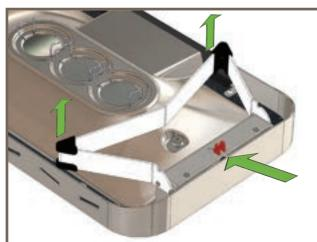
2. To unfold the legs, firstly move and hold the locking levers (1) in the direction shown by the arrow cut-outs. Then fold the legs (2) to the upright position in the direction of the green arrows.
